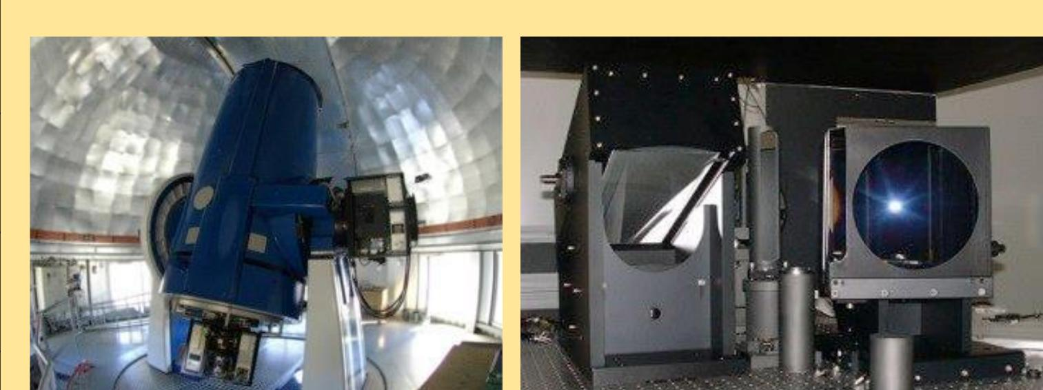
The 1.2-m Mercator Telescope(left) with HERMES Fibre-fed echelle spectrograph(right), Roque de los Muchachos Observatory, La Palma, Spain.
