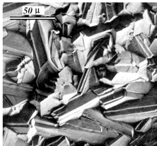
Fig. 2. Optical photograph of the diamond surface showing non-oriented crystallites
