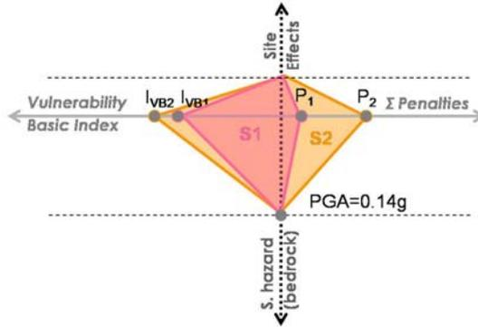
Figure 4 - The horizontal plane of the risk representation according to the method used in Liège for the two houses of our example. There is a relation between the surface of the quadrilateral, defined by hazard and vulnerability, and the damage rate. This rate is calculated following linear relationship (1) that often leads to overestimation.
