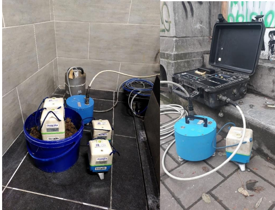
Figure 5 : Left: Lab-based instrument test of two nodes each based on a tripod or with a spike in a sand-filled bucket next to a classical LE3D/5s (blue pot) seismometer and the well calibrated Guralp sensor of the UCCS permanent station (gray cylinder). Right: Comparison of Lennartz LE3D/5s with city shark digitizer and tripod-based node sensor close the Wiels Cultural Centre in Forest (Brussels).
