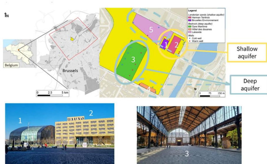
Figure 22: Location of the Tour & Taxi site, and the different buildings. Buildings 1 and 2 are pumping and reinjecting groundwater in the Cenozoic aquifer, buildings 3 to 5 in the Cambrian aquifer. The geothermal systems of buildings 4 and 5 have not yet started to be operational.
