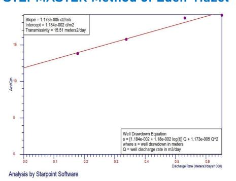
✓ Interpretation with Barker (1988) solution of first pumping phase of step-drawdown test
