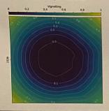
**Filters uniformity** The small pupil design is sensitive to the uniformity of the transmittance. This is not accounted for yet in L2 data but amounts to less than 10% across the FOV.
