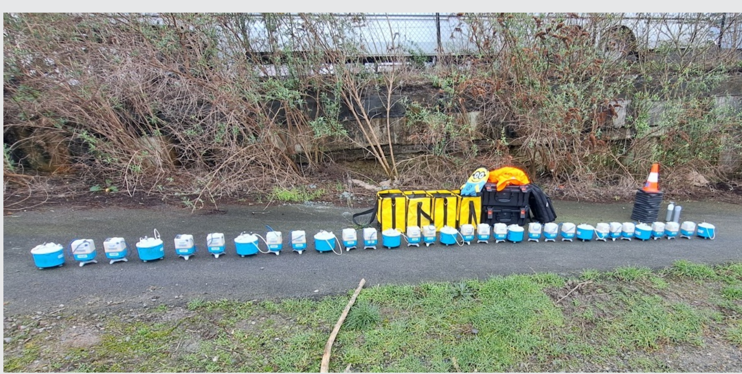
SmartSolo® IGU-16HR and IGU-BD3C-5 seismic sensors used for geophysical prospection below a bridge in Halle (BE)
