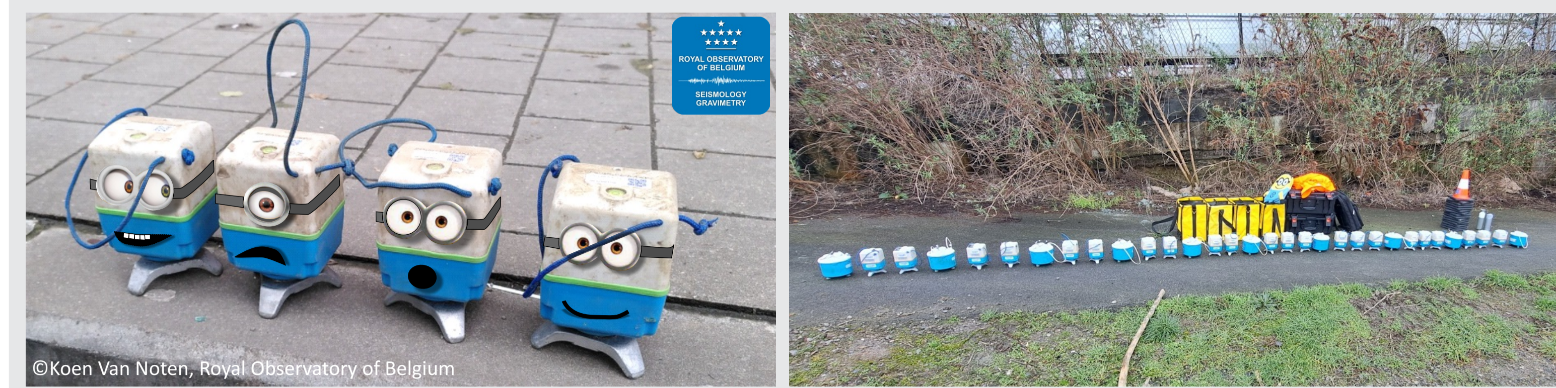
SmartSolo® IGU-16HR 3C connected to standard battery tripods during an urban seismology campaign in Brussels
