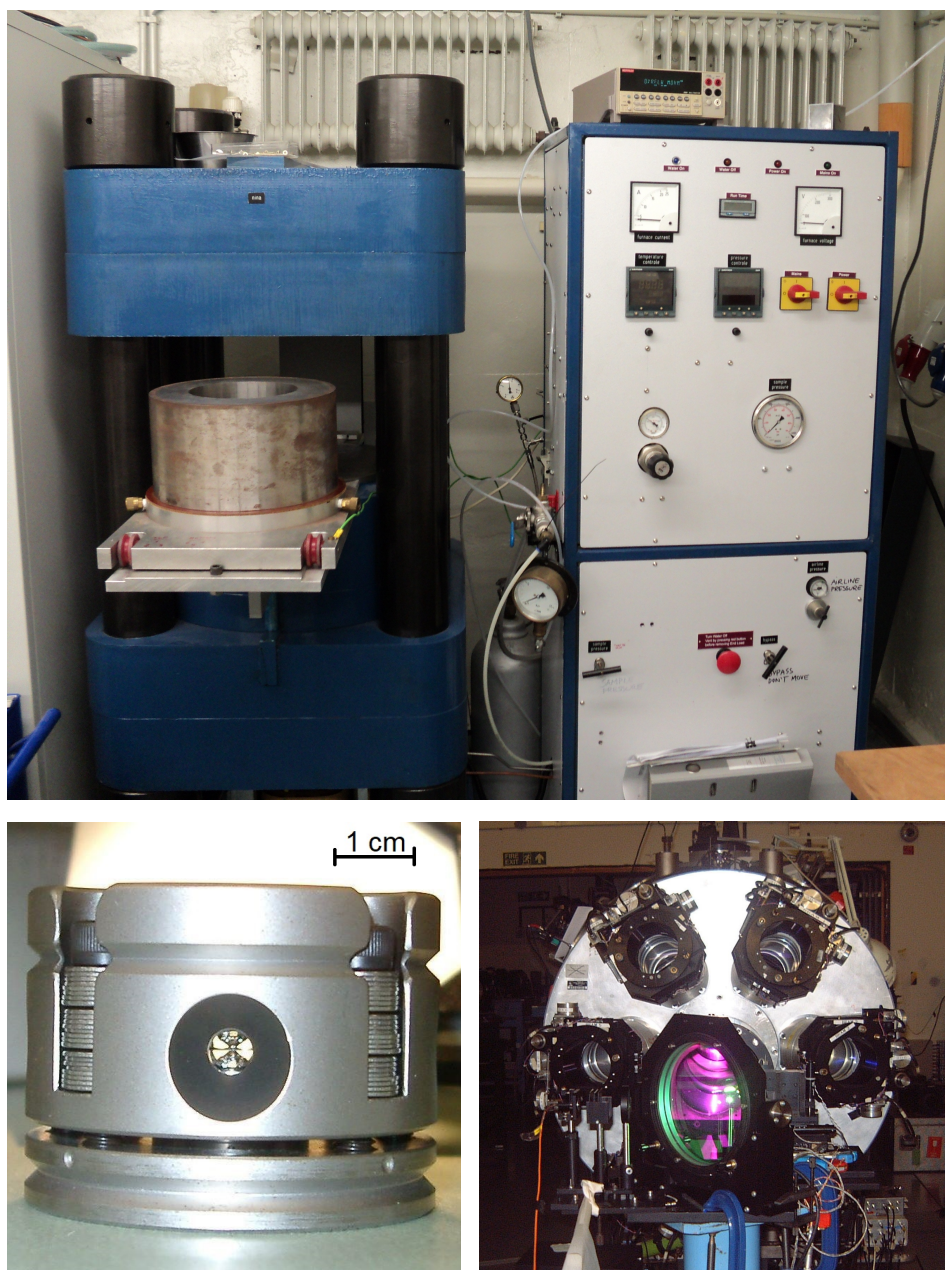
Figure 1.10: Top: Multi-anvil device (Nina) in the High-Pressure-Temperature Laboratory, Vrije Universiteit Amsterdam. Bottom-left: Diamond-anvil cell at the Laboratory for Mineral Physics, University of Chicago. Two gem-quality diamonds inside the cell are visible through the hole. Bottom-right: Laser-driven shock wave experiment set up at the High-Pressure Mineral Physics Laboratory, New Mexico State University.
