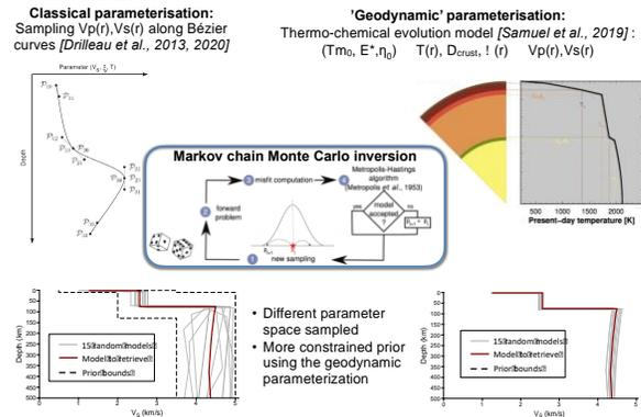
Figure 1: Schematic representation of a classical [11] (left) and a geodynamic parameterization [10] (used here) to infer Mars' seismic structure via Monte Carlo Markov chain inversion of seismic data.
