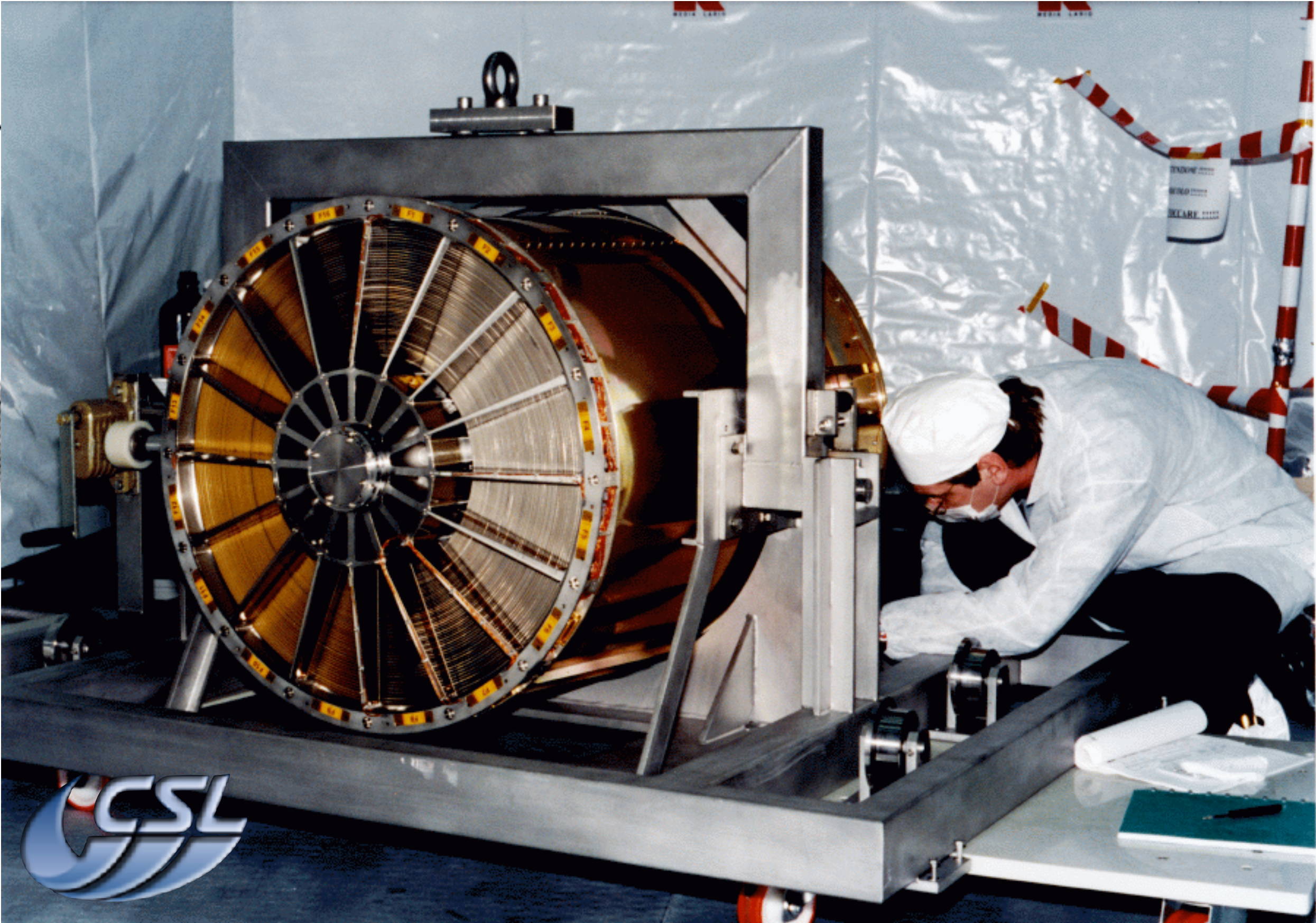
XMM mirrors during tests at Centre Spatial de Liege
