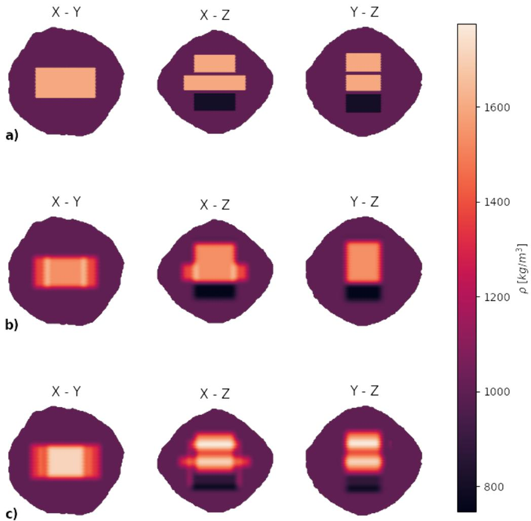
**Figure 1.** Interior density models, shown via sections along 3 planes perpendicular to the body axes and containing the origin: a) Ground truth; b) Solution from noise-free data; c) Solution from data with 1% noise
