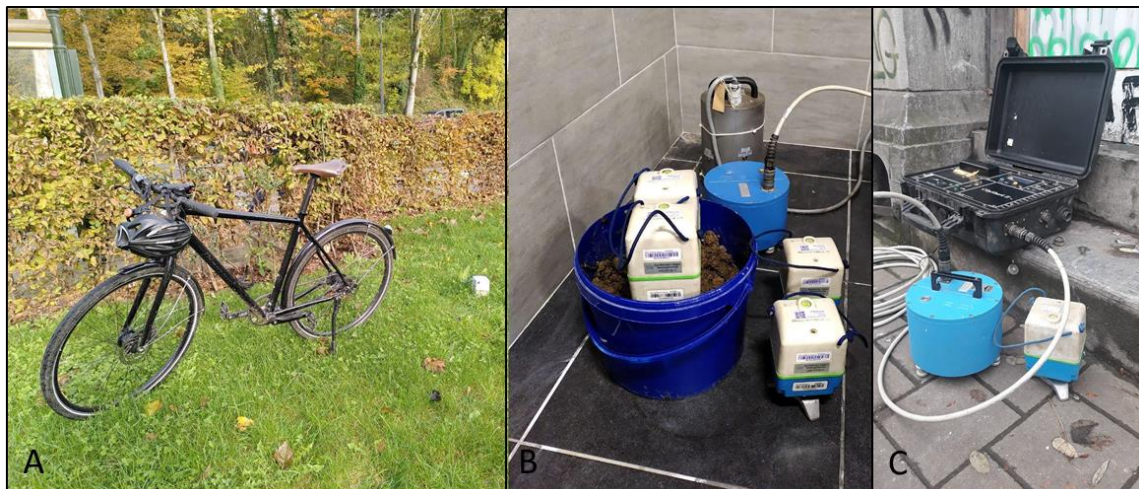
Fig. 1 - A: 3C lightweight sensors are transported for urban investigations with all means of transport. B: Set-up of lab-based instrument test, top : surface sensor of UCC seismic station, blue : Lennartz 3D/5s, four SmartSolo sensors with two sensors ( left ) with spikes in a sand-filled bucket and two sensors ( right ) on tripods. C: Ambient noise measurements on a paved footpath next to the abandoned Brasserie Wielemans in Forest (Brussels). Co-location of a 3C sensor installed on tripods and a Lennartz - Cityshark setup.
