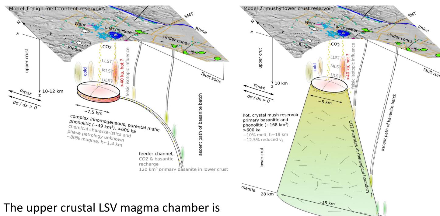
predicted in 4-10 km depth, but has not been detected with geophysical data so far. The sketches show two hypothetical models how the reservoir system may look. A dense seismic network and novel analysis methods are
