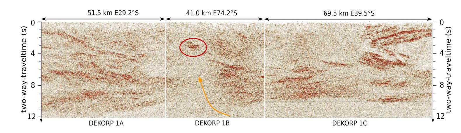
Reprocessed reflection seismic profiles (DEKORP 1, 1987) crossing the West Eifel at the Kelberg magnetic anomaly. Beneath Kelberg a bright spot is resolved (old reservoir). The youngest maar (Ulmen) is at the center of the profile. The transparent zone beneath Kelberg indicates a hot region and presence of melts (mush reservoir?)
