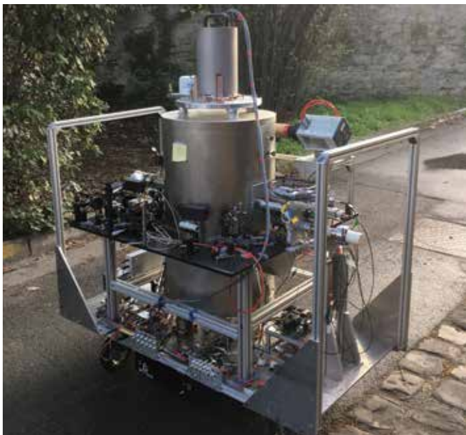
This absolute gravimeter developed by the SYRTE (Time and Space Reference Systems) department at the Paris Observatory uses ultracold-atom technology to make high-precision measurements of gravity. Credit: Sébastien Merlet, LNE-SYRTE
