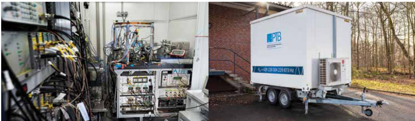
The transportable optical clock of the Physikalisch-Technische Bundesanstalt (PTB), the National Metrology institute of Germany (left) is housed inside a trailer (right). Credit: PTB Braunschweig, CC BY 4.0 ( bit.ly/ccby4-0 )
