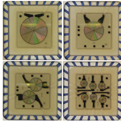
Fig. 4: MSM-AlN photodetectors of several sizes (1.1 to 4.3 mm diameter).
