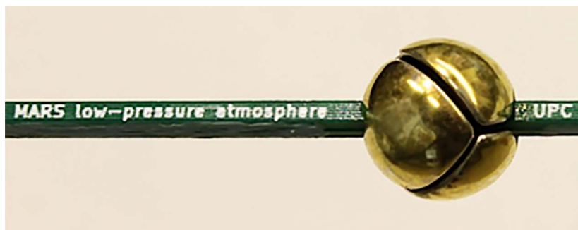
Fig. 1. Photograph of the 4-sector spherical sensor (10 mm diameter), before being wrapped and inserted into the regolith simulant
