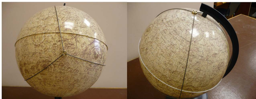
Fig. 1. A model of a network of observation points on the surface of the moon that coincides with the vertices of the tetrahedron inscribed in the lunar sphere
