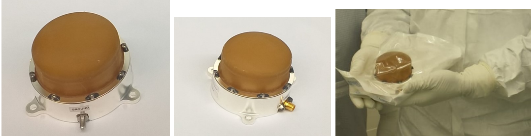
Figure 7: Pictures of the receiving (Rx) (left) and transmitting (Tx) antennas (center), and Tx when ready for pattern measurement, after planetary protection process (right).
