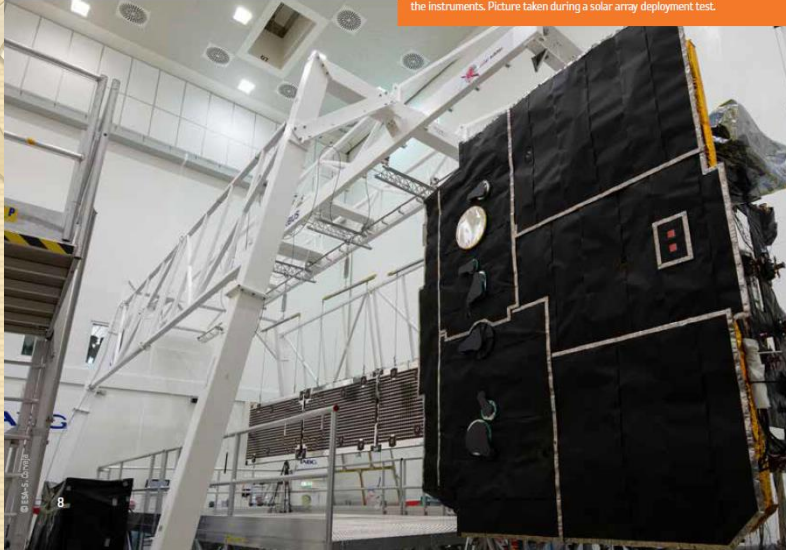
Solar Orbiter's 'SolarBlack' heatshield, with covers to protect some of the instruments. Picture taken during a solar array deployment test.
