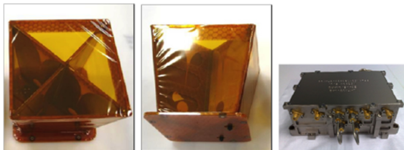
Fig. 11. SSR antenna and electronics box.
