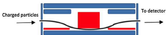
Fig. 19. ChaPS Bessel box geometry. Red are the electrodes that hold the voltage and blue are at ground. (For interpretation of the references to color in this figure legend, the reader is referred to the web version of this article.)
