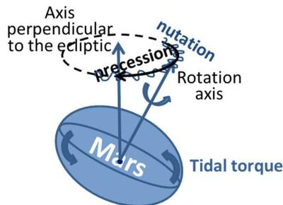
**Figure 2:** Representation of precession and nutation of Mars.
