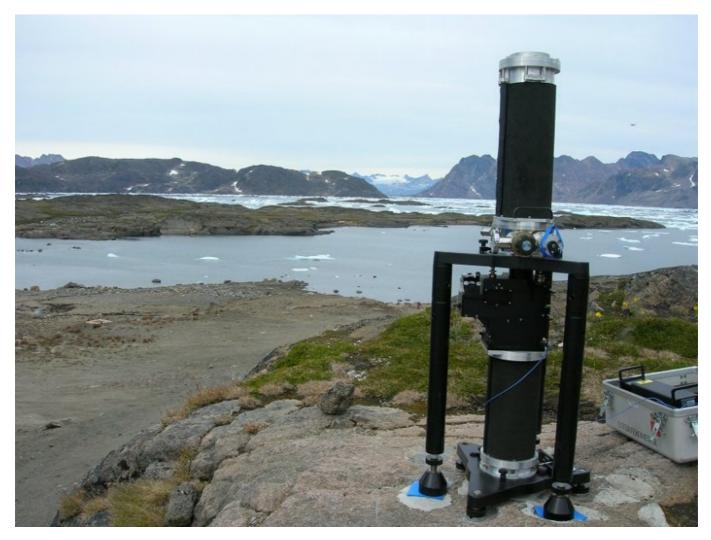
A FG5 absolute gravimeter measuring ice mass changes in Kulusuk, East Greenland.
