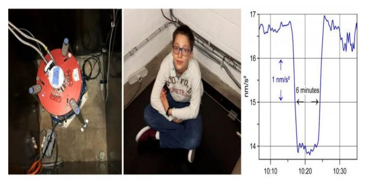
Left: A superconducting gravimeter installed in a shaft at the Rochefort station, Belgium. Center: A 13-year old boy, weighing 45 kilograms, sat with his navel 1 meter above the instrument. Right: The gravitational effect of the boy sitting for 6 minutes: his mass induced a decrease in gravity of 0.28 billionth of *g*. Credit: Royal Observatory of Belgium/Van Camp et al, 2017 (http://onlinelibrary.wiley.com/doi/10.1002 /2017RG000566/full), Figures A4d and A7
