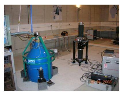
Superconducting (blue) and absolute (black) gravimeters measuring at Conrad Observatory,
