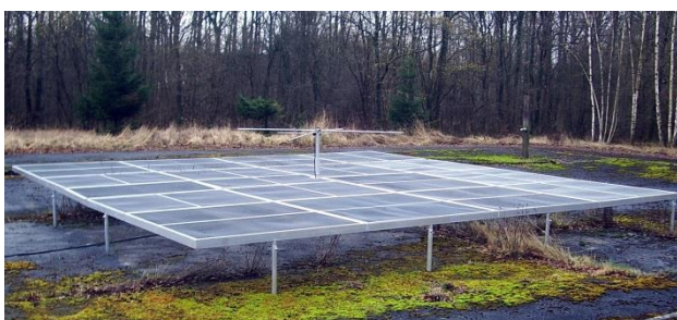
Figure 1 – BRAMS beacon radiating system in Dourbes, Belgium.
