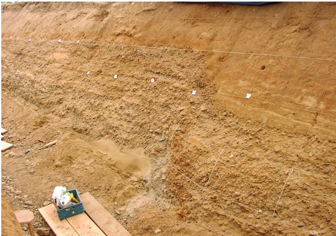
Fig. 56– Photograph of northwestern wall of trench Rotem-2 in the Belgian Maas valley, showing the Geleen fault vertically displacing the top of the late Weichselian terrace and overlying eolian sands and silts by 0.75–1 m.
