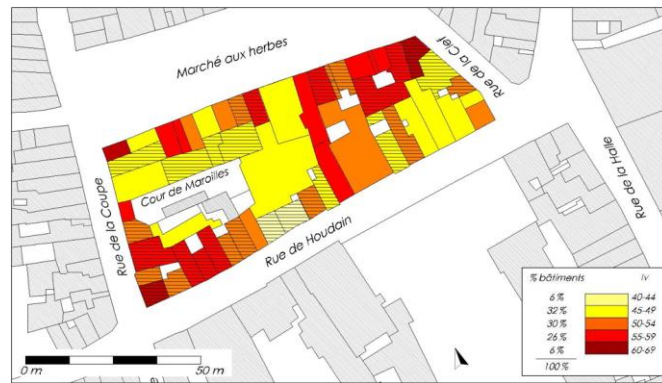
Figure 3 – Determination of the vulnerability index V_i in a part of the historical centre of Mons [5]
