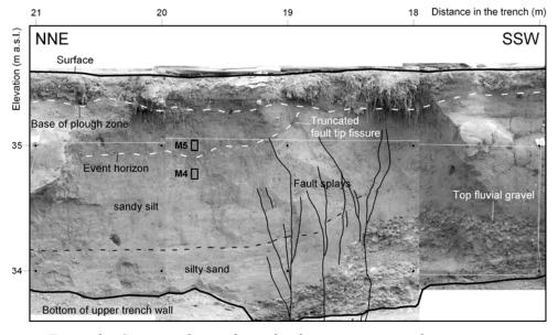
Figure 3 – Stratigraphic evidence for the most recent surface-rupturing earthquake in a paleoseismic trench across the Geleen fault near Rotem.
